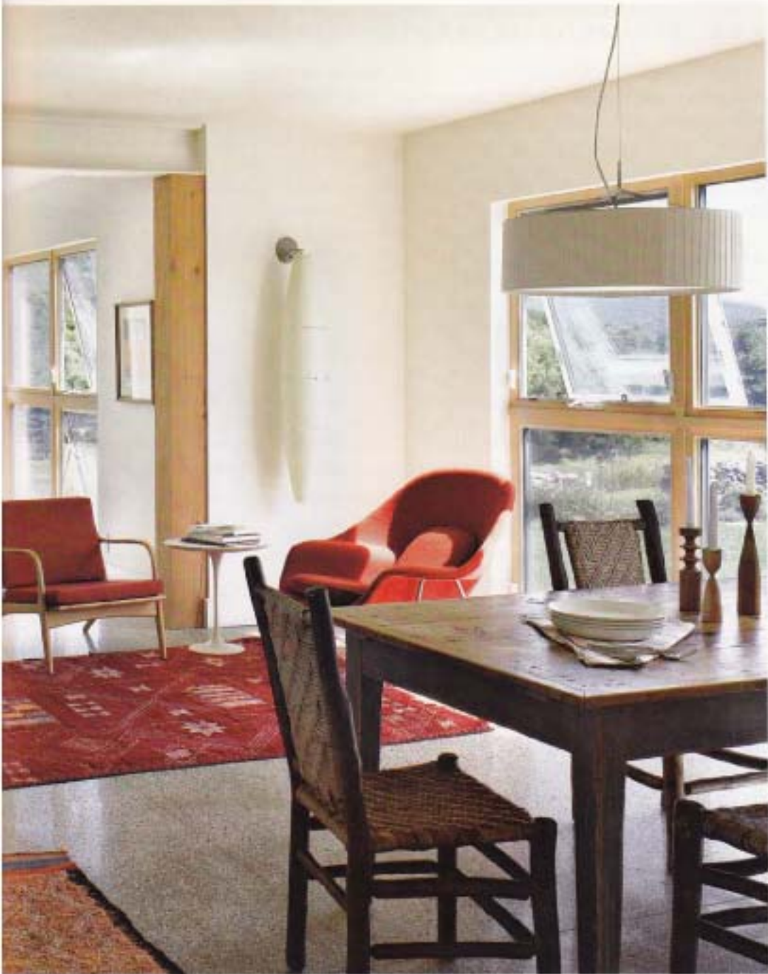
A radiant-floor system provides heat. The thermal mass of the polished concrete slab is an energy bank that stores heat and helps even out sudden changes in indoor temperature.
